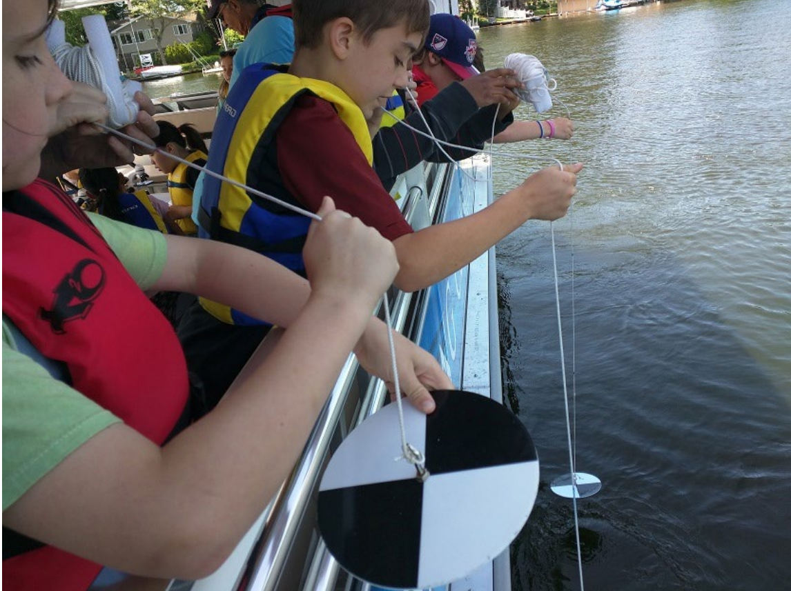
Guests aboard the Lake Hopatcong Floating Classroom take part in scientific experiments like water clarity testing with secchi disks.
